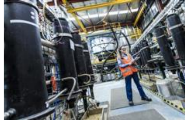
Column leaching facility
