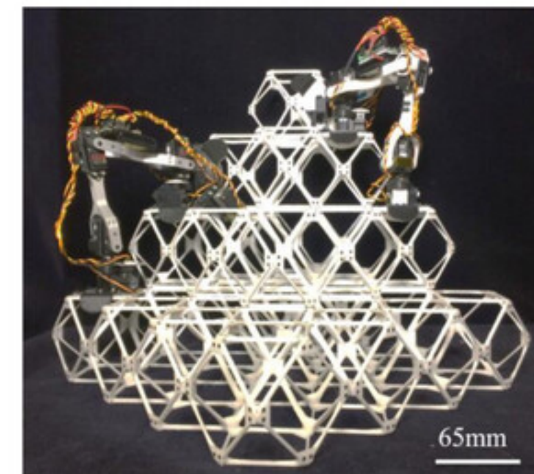
Figure 1: Mobile robots which assemble a discrete cellular structure. This pyramid structure consists of 30 cuboctahedral voxels.
