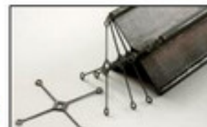
BUILDING BLOCKS Thin slices of carbon fiber composite can link together to build lightweight lattices that could one day form the framework of airplanes and spacecraft. Image © CC-BY-NC-SA Kenneth C. Cheung
