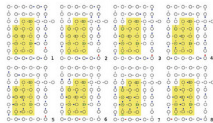
Fig. 4 Steps in the calculation of Fibonacci numbers with an ALA one-bit full adder
