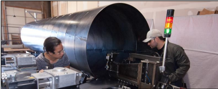
KTS 1/7 scale working machine to produce test towers
