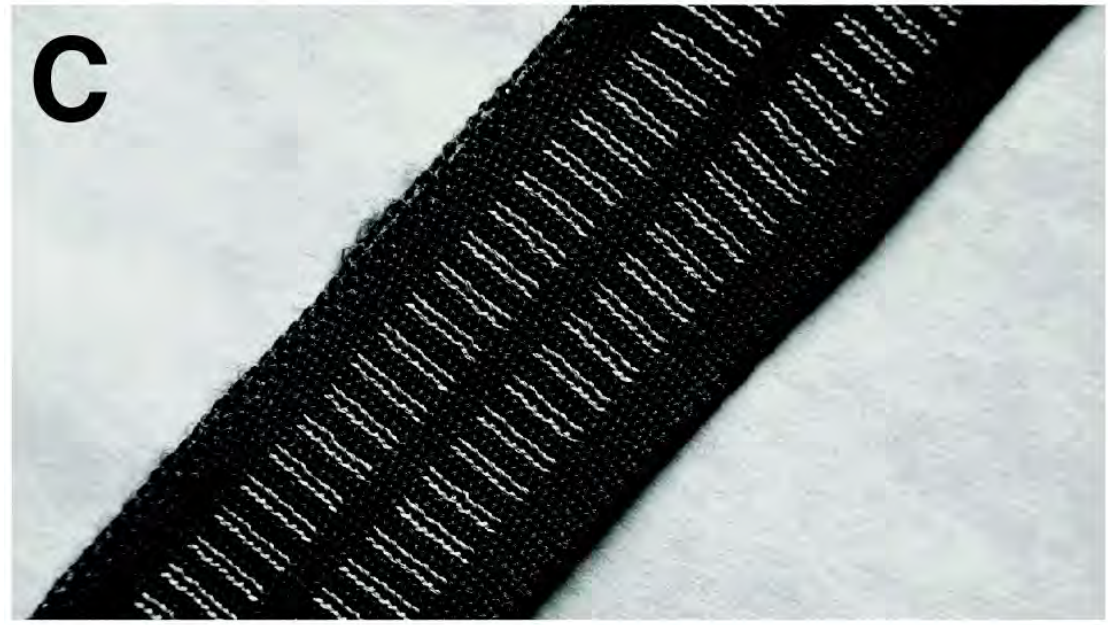
(A–C) Belt rheostat illustration, knit design, and sample photograph. (D–F) Tablecloth rheostat illustration, knit design, and sample photograph. (G–I) Stretch sensor illustration, knit design, and sample photograph. (J–L) Displacement/pressure sensor illustration, knit design, and sample photograph.
