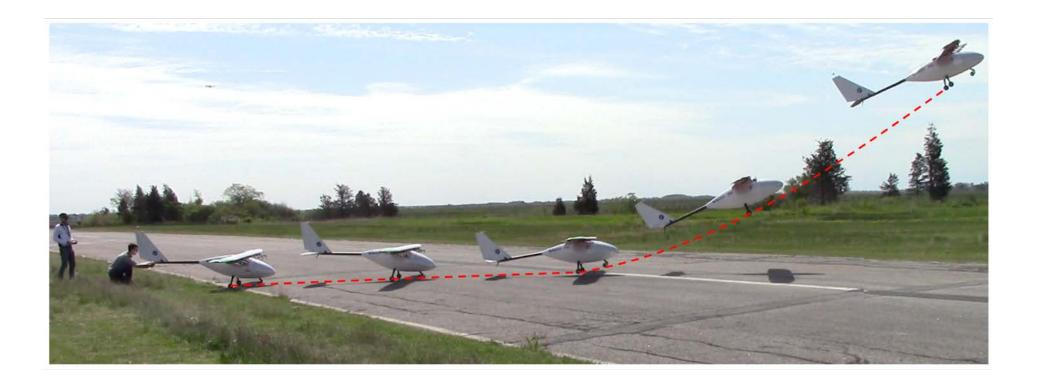
Flight demonstrator shows that high lift ( $C_L > 10$ ) is achievable in real-world flight environment but that there are control challenges to be addressed.
