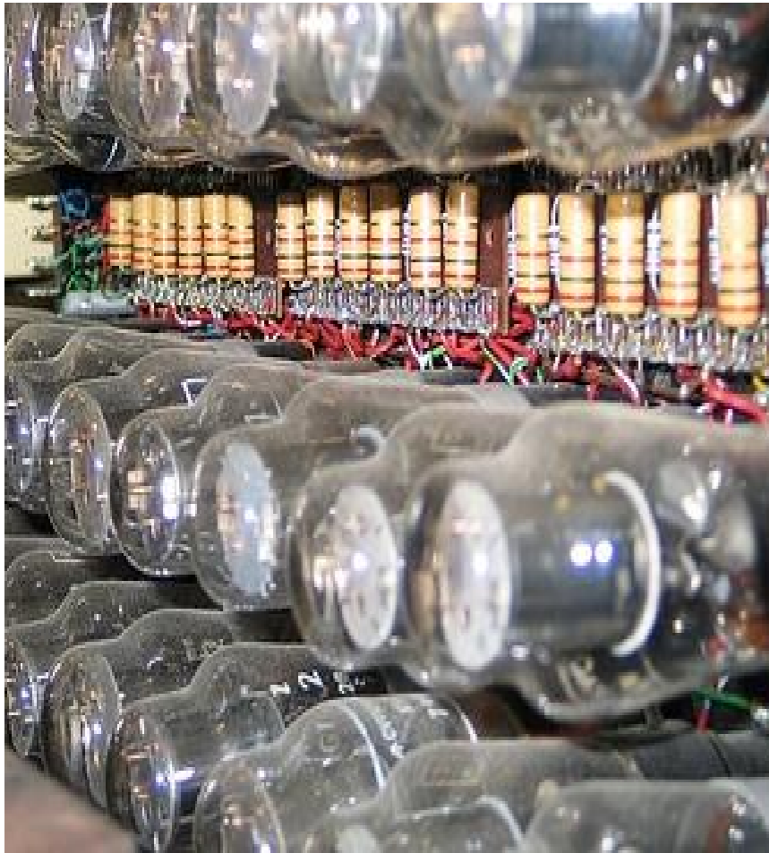
Thermionic vacuum tubes in Colossus Mark 2 (1940s) (Bletchley Park Museum)
